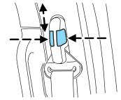
pull down on the height adjuster to make sure it is locked in place.
